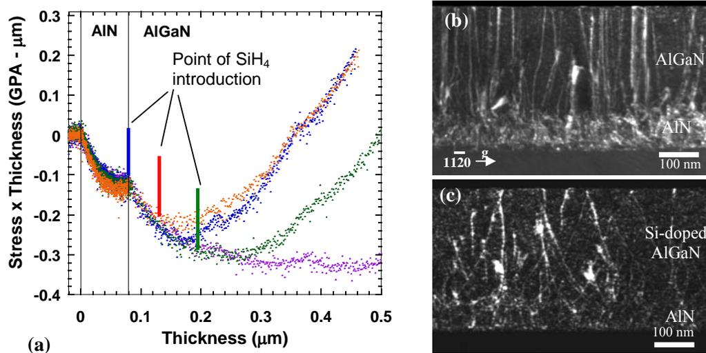
**Figure 2.** (a) Stress-thickness vs. thickness plots for Si-doped  $\text{Al}_x\text{Ga}_{1-x}\text{N}$  layers grown with  $\text{SiH}_4$  introduced at different layer thicknesses as indicated in the figure. Weak beam dark-field cross-section TEM images obtained using 112-0 diffraction conditions for (b) undoped  $\text{Al}_x\text{Ga}_{1-x}\text{N}$  and (c) Si-doped  $\text{Al}_x\text{Ga}_{1-x}\text{N}$  in which  $\text{SiH}_4$  was added at the beginning of growth.
